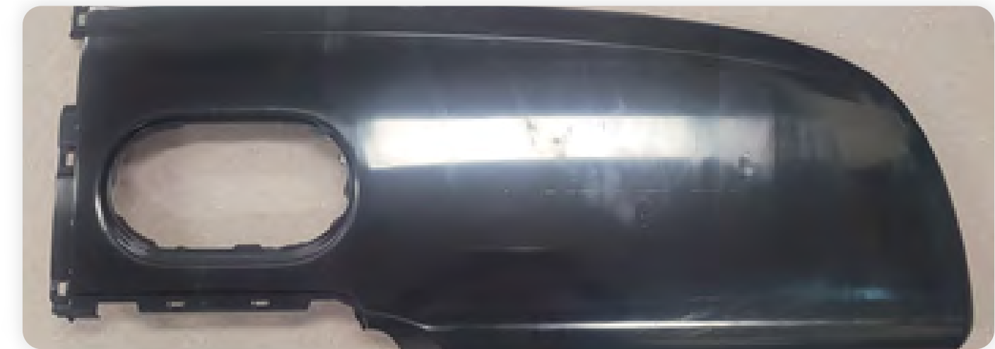
Crash pads made with biodegradable PC composites
